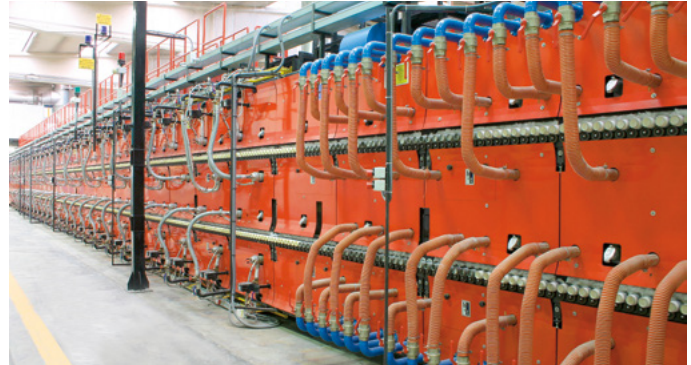
Roller hearth kiln in the ceramics industry
